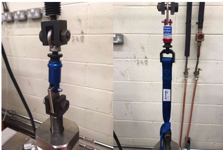
Photo Ref. 5693 Large O-Ring Test Set-Up Photo Ref. 5693 Large Lead Test Set-Up
